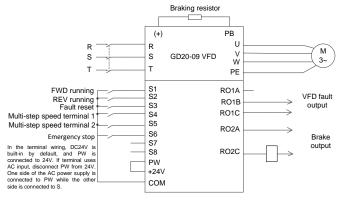
Figure 4-3 Wiring for horizontal moving
