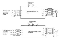
Figure 3-3 Wiring diagram of main circuit
