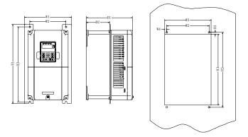
Figure B-6 Flange mounting diagram of 7.5–37kW VFDs
