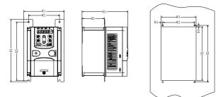
Figure B-5 Flange mounting diagram of 5.5kW VFDs
