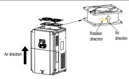
Figure 7-2 Fan maintenance for 5.5kW and higher VFD models
