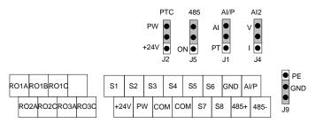
Figure 3-10 Control circuit terminal diagram of 5.5kW-37kW VFD models
