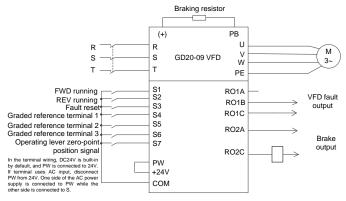
Figure 4-6 Wiring for graded reference operating lever
