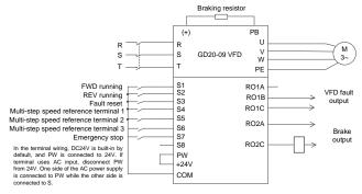
Figure 4-7 Wiring for multi-step speed reference
