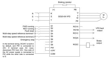
Figure 4-1 Wiring for open-loop vector control
