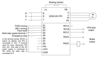
Figure 4-4 Wiring for the conical motor
