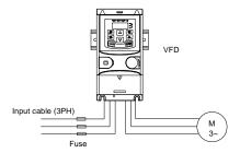
Figure 3-16 Fuse configuration
