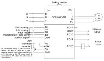
Figure 4-5 Wiring for analog reference operating lever
