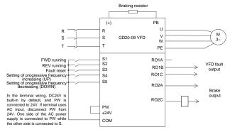
Figure 4-8 Wiring for motor-actuated potentiometer
